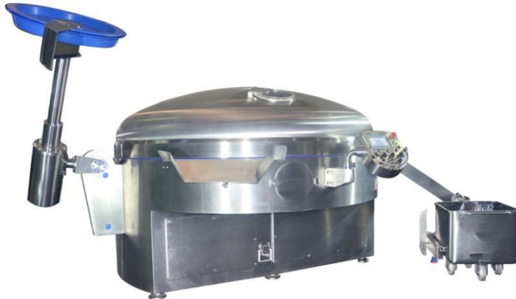
750 Ltr. Vacuum Bowl Cutter with loader, unloader
