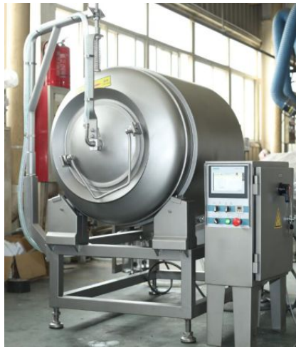
Vacuum Tumbler KVT 500 with cooling
