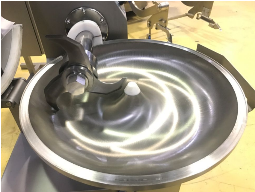
Bowl stainless steel with knife head and 3 knives
