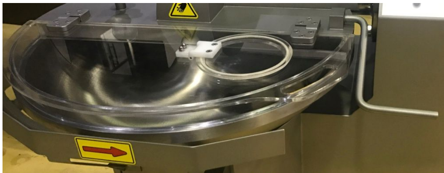
Noise reduction Lid with standard spice flap
